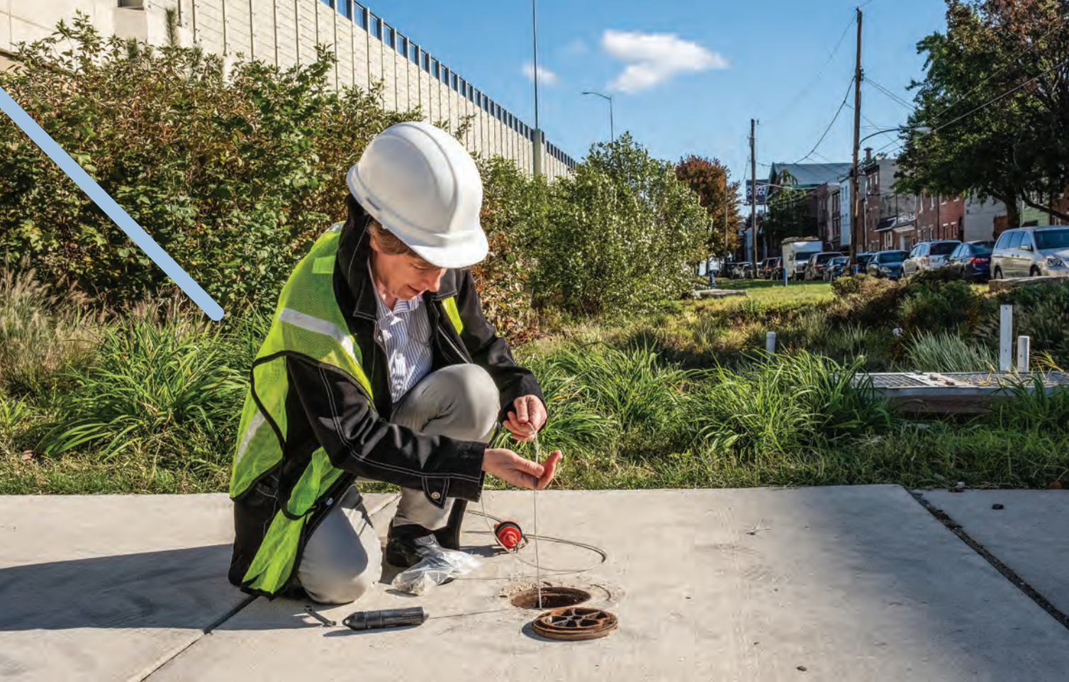
To measure the fluctuating depth and chemical concentrations of the groundwater near the interstate, Toran uses a battery-operated device called a logger.
