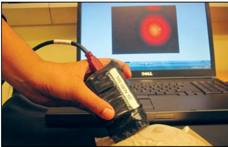
A tactile imaging sensor developed by Temple Associate Professor of Electrical and Computer Engineering Chang-Hee Won can emulate human tactile sensation, which may help doctors get early information about lesions and tumors.
