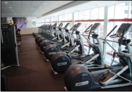
The Fitness Mezzanine at Pearson-McGonigle Hall includes 12 cardio machines that are tied to a Re-Rev system, which recycles kinetic energy from workouts by sending power back to the building grid. Bri Bosak
